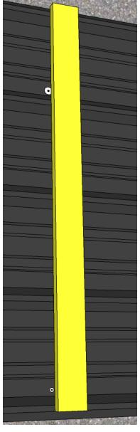
edge across the panels at each of these rows and mark ribs 2 and 3 (See Figure 8). This method tends to visually catch errors in marking. It is not necessary to mark rib 5 because it is the under-lap and it is not necessary to put a screw by it. Remember that if you drill wrong you've probably ruined the whole stack.
